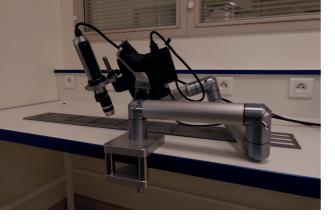
THE 3D DIGITAL MICROSCOPE (VHX-7000) COMBINES, IN ONE SINGLE SYSTEM, FUNCTIONS OF OBSERVATION, IMAGE CAPTURE AND MEASUREMENT. IT OFFERS HIGH QUALITY IMAGES ALLOWING TO REDUCE THE TIME SPENT ON CONTROL.
